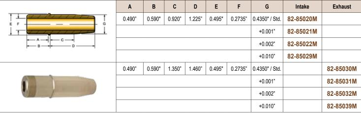
These Manganese guides are easily reamed, and then can be delicately finished with our high quality ball hones. Now, with any battery operated or electric drill you can ream and hone manganese valve guides in less time and in the absence of expensive honing equipment required to properly size "tough" Nickel Bronze guides.
